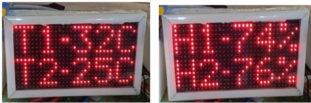
Fig 12. P10 board display of the monitoring system
