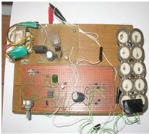
Fig.11 Complete diagram of power harvesting system
