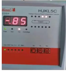
Fig 16. Initial Power Factor Value in Reactive Power Compensation Controller
