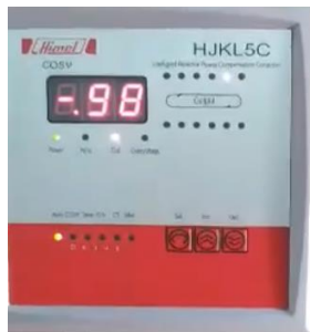
Fig 17. Target Power Factor Value in Reactive Power Compensation Controller
