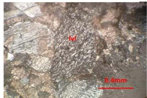
(Fig.14) Photomicrographs showing the volcanic lithic grain with lathwork texture (Ivl) of the Zigyaing Formation (Under X.N)
