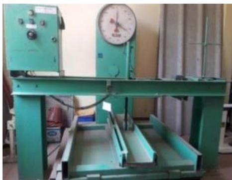
Fig 5 Bending strength test machine
