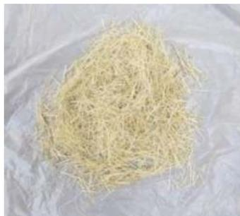
Fig 1 Bamboo fibre
