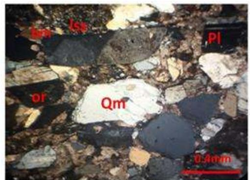
(Fig.8) Photomicrograph showing the monocrysstalline quartz (Qm), orthoclase feldspar (or), plagioclase feldspar (pl), and biotite mica (bm) of the Zigiaying Formation (Under X.N).
