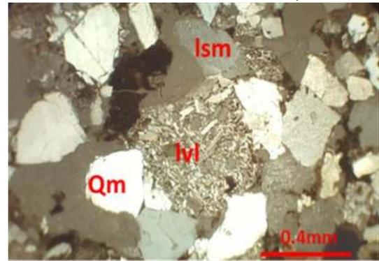
(Fig.12) Photomicrograph showing monocrystalline quartz (Qm), volcanic lithic grain with lathwork texture (Lvl), and sedimentary rock fragment (Lss) (Under XN)
