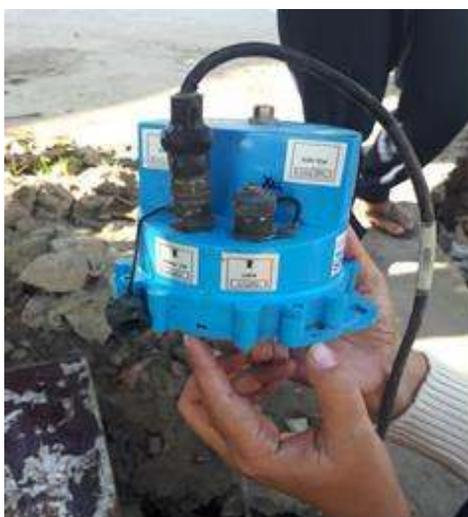
Fig 2. Water pressure sensor
