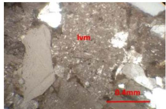
(Fig.13) Photomicrographs showing the volcanic lithic grain with microlithic texture (Ivm) of the Zigyaing Formation (Under X.N)
