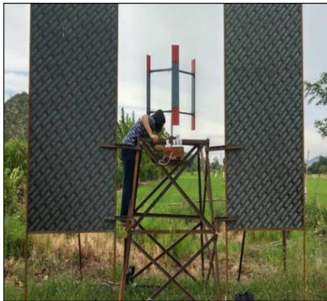
Fig 6. Diffuser integrated turbine assembly
